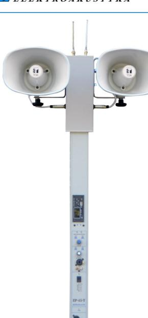
Modern portable sound system ZP-45-T is designed for sounding processions, pilgrimages, open spaces. Includes 3 x 3.5 speaker, 2 horn speakers, radio transceiver set, amplifier and battery. The amplifier operates in class T, characterized by great efficiency, which allows for extended operating time. The kit includes a battery charger, harness and a stand.
